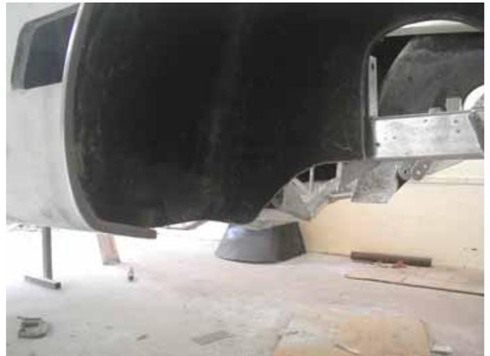
**17.** Mark the front and rear wheel arch lips at around 16 to 19 mm. This can be done with a scribing block or a wood working mortise gauge or with a spacer block and a scribe. You will also need to trim the lower edge of the inner wheel arch to clear the lower thrust arm, (this can be measured from the chassis or marked from a card pattern and trimmed on final fitting of the body to the chassis).
