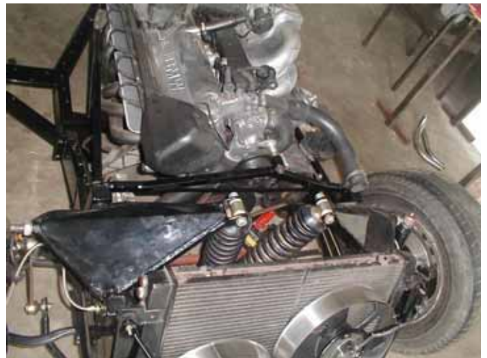
Engine brace to prevent rocking under heavy use! (As we plan to do with this car)
