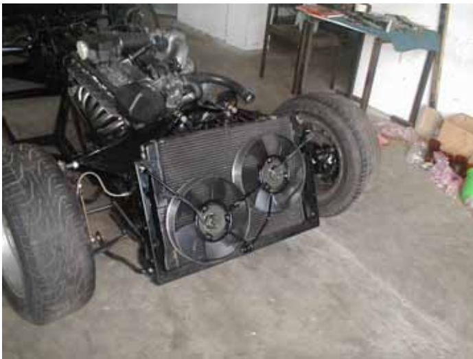
E28 535i radiator and two Toyota fans On fabricated frame and cowls
