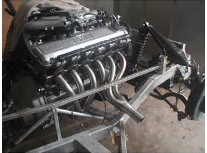
Exhaust manifolds in position (side pipes) M20 block 525i
