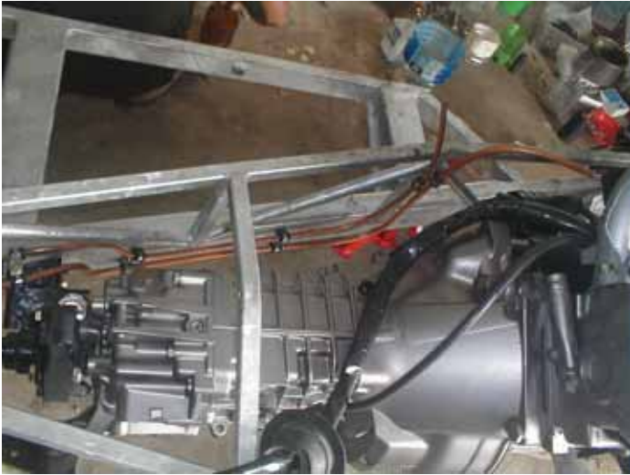
Fuel pipes ready for connection
